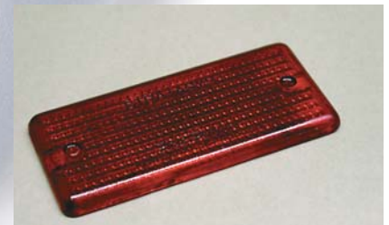
Figure 4: Finished model with clear coat (optional) The translucent red color of the finished model is perfect for this tail-light lens. Clear coat spray protects the finish and adds luster to your showpiece
