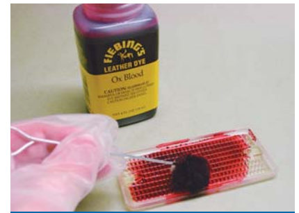
Figure 2: Apply aniline dye Aniline dye is applied to the model by brushing (shown), or dipping
