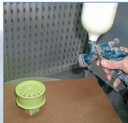
Figure 7. Apply Final Paint.
