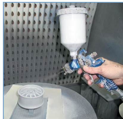
Figure 6. Apply Primer Paint.
