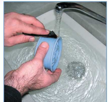
Figure 2. Wet-sanding. Wet-sand the model with 320-grid sandpaper.
